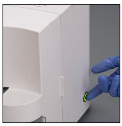
**Fig. 31:** Press the On/Off button to switch on the analyzer
