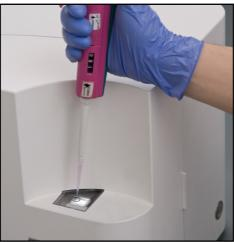
**Fig. 36:** The backlighting under the see-through plastic cuvette helps you guide the tip of the pipette for fast and efficient work
