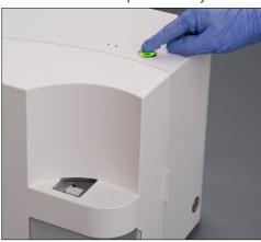
**Fig. 34:** The Start button on the top of the analyzer is the only interface element you need: press it once and the system feeds a cuvette into pipetting position.
