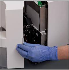
**Fig. 32:** Open the analyzer door to access the cuvette holder slot
