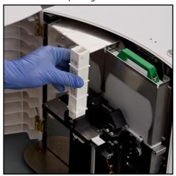
**Fig. 33:** Slide a cuvette holder into the holder slot, then remove the tape from the bottom before you start a measurement
