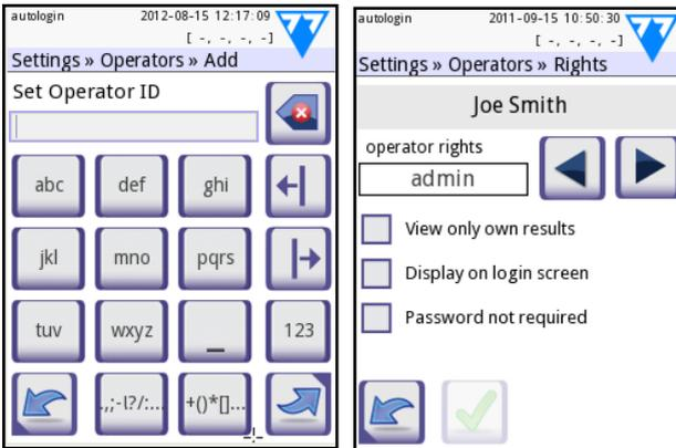
**Figure 47:** *The Operators » Add and the Operators » Rights screens*
