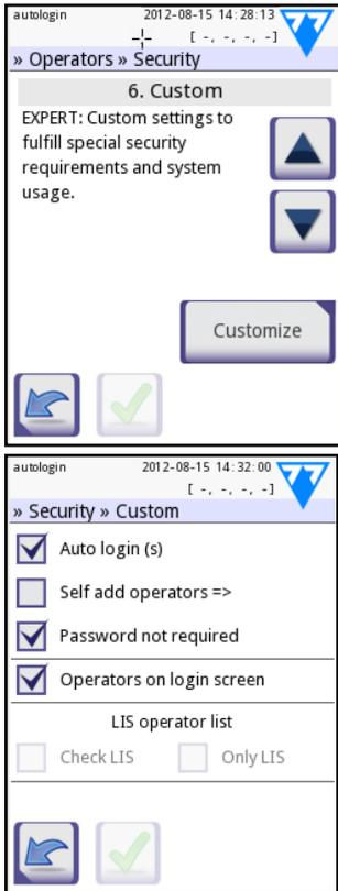
**Figure 46:** *The sixth Security screen and the Operators » Security » Custom screen*
