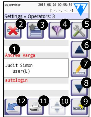
**Figure 45:** The *Settings » Operators* screen with its function buttons labelled
