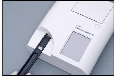
**Figure 3:** Inserting the test strip tray
