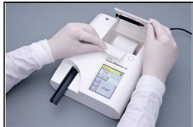
**Figure 4:** Loading the printer
