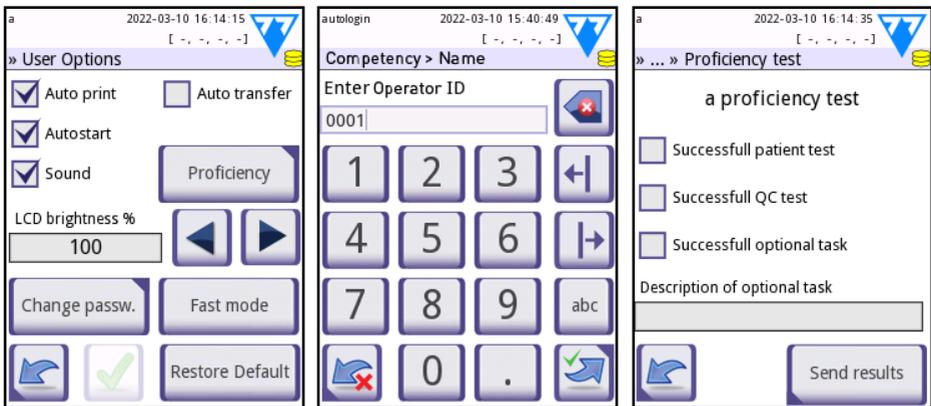
**Figure 36:** Proficiency test feature
