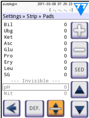
**Figure 40:** The *Settings » Strip » Pads* screen with an example of invisible analytes
